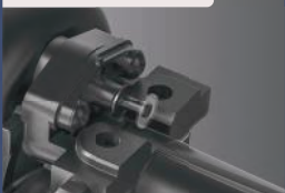
Clutch wear indicator
